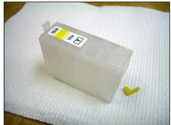
Turn the cartridge over and use a syringe needle to pierce a small hole in the film over the ink exit port. Do not push the needle into the cartridge – just use enough pressure to make a hole in the film. Do not try and remove the film from the port. After making a hole in the film, turn the cartridge back upright.
