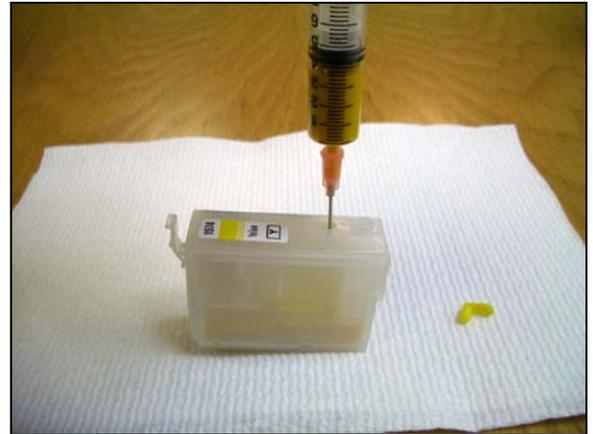
Refill the syringe with another 10 ml of ink and continue injecting ink into the cartridge. This will nearly fill the cartridge. Insert the colored bung back into the ink fill hole and remove the white bung from the air vent hole. Use paper towel to wipe up any ink that may be on the top surface of the cartridge or around the fill hole.
