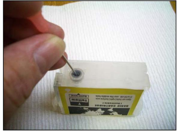
Using a clean syringe with needle fitted, draw up 10 ml of ink from the correct color ink bottle. Double check that you are using the correct color ink corresponding to the color of the cartridge – filling the wrong color ink into a cartridge will mean that the cartridge has to be replaced. Gently inject the ink into the cartridge until the syringe is empty, as in this picture.
