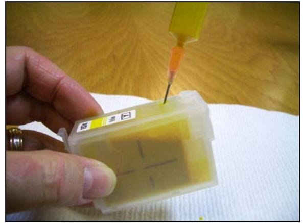
Fill all the cartridges you intend to install at this time. Use a clean syringe, needle and end adaptor for each ink color and always double check that you are filling the correct color ink into the correct color cartridge.
