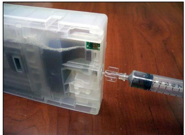
syringe between colors so that no cross contamination of colors can occur. Once you have removed the air from all the cartridges, install the cartridge or cartridges into the printer just as you would with normal cartridges. **Remember to remove the rubber bung from the air vent hole on each cartridge as you install them.** The printer is now ready to be used.
