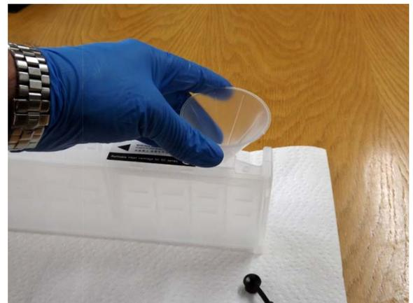
After you have filled the cartridges, you will need to extract a small amount of air from each refillable cartridge that gets trapped during the initial filling process before you first install the cartridge in the printer. Failure to do this will mean that this trapped air will eventually make its way to the print head and cause some nozzle drop outs during printing.
